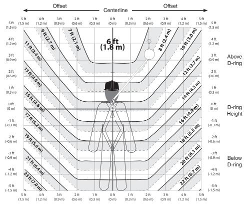
**EXAMPLE:** With the SRL-LE anchored 4 feet above the users D-ring and the user works 2 feet away (offset) from directly overhead (centerline), the required clearance is 7 feet (2.1 m) from the working level to the nearest obstruction below.
