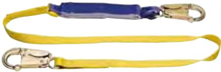
These lanyards utilize a packed deceleration device (shock pack) designed for controlled tearing action to reduce fall arrest forces.
