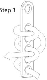
3. On same side of the product, feed rope through other loop located between holes 2 & 3.
