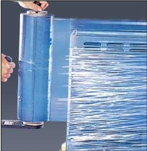
Secures and protects pallets of large metal parts for shipment or storage.
