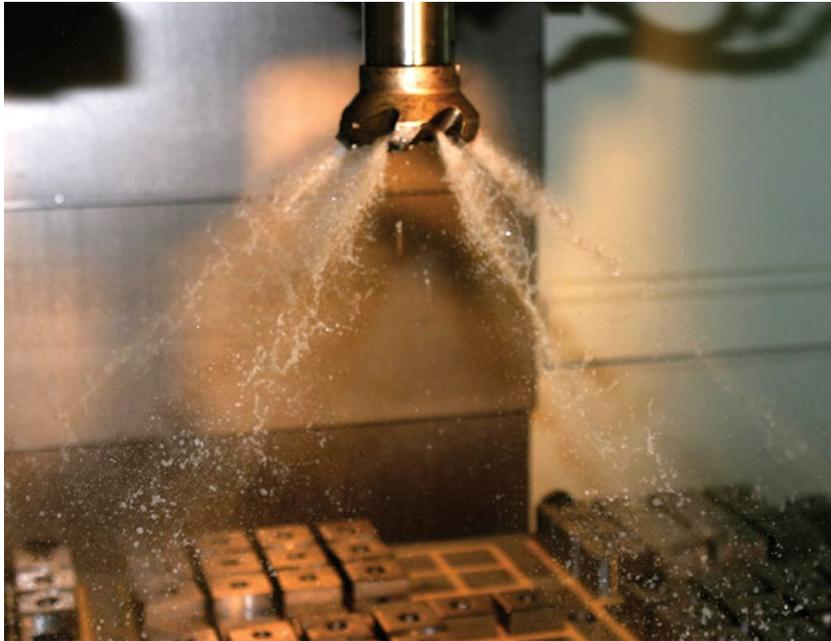
CoolBLAST arbor screw provides coolant path.
