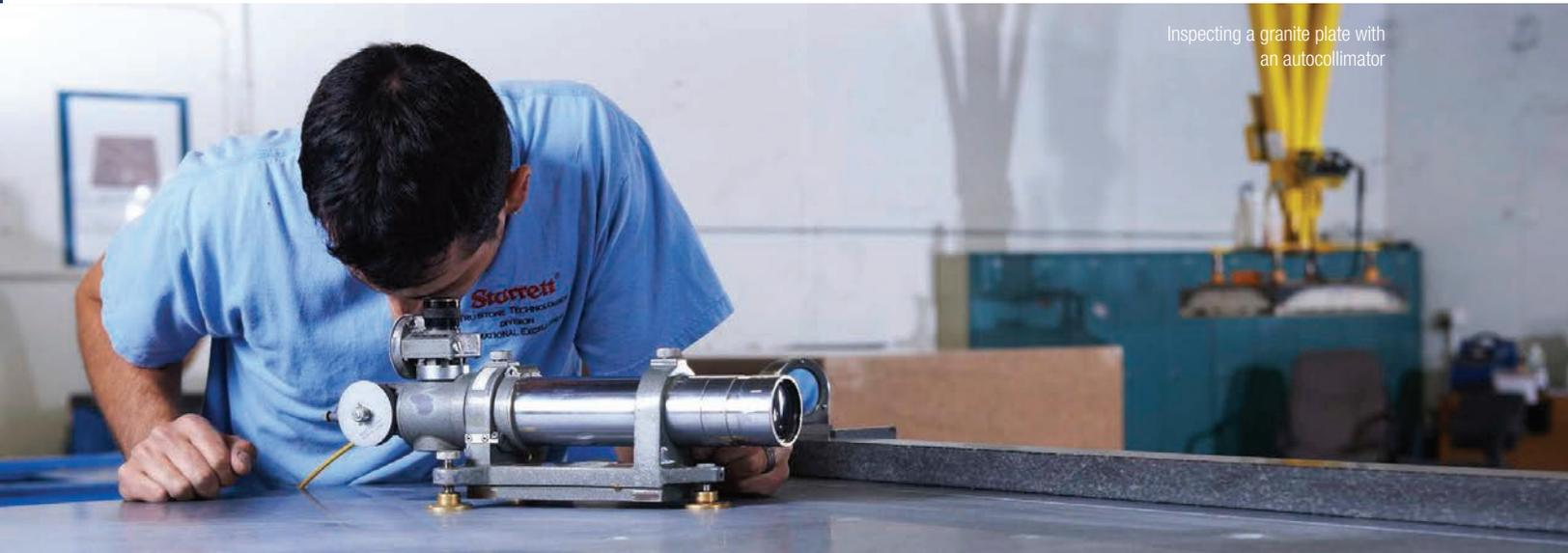
Inspecting a granite plate with an autocollimator
