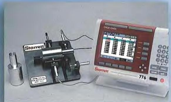
The 776 accepts multiple gage inputs simultaneously – invaluable for applications such as this Starrett special gage fixture
