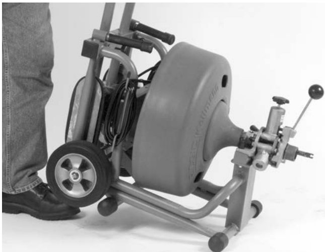
Figure 7 – Releasing Kickstand Bar
