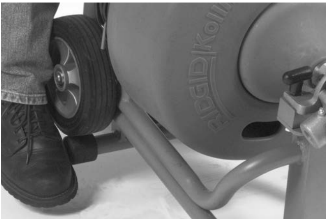
Figure 6 – Setting Kickstand Bar
