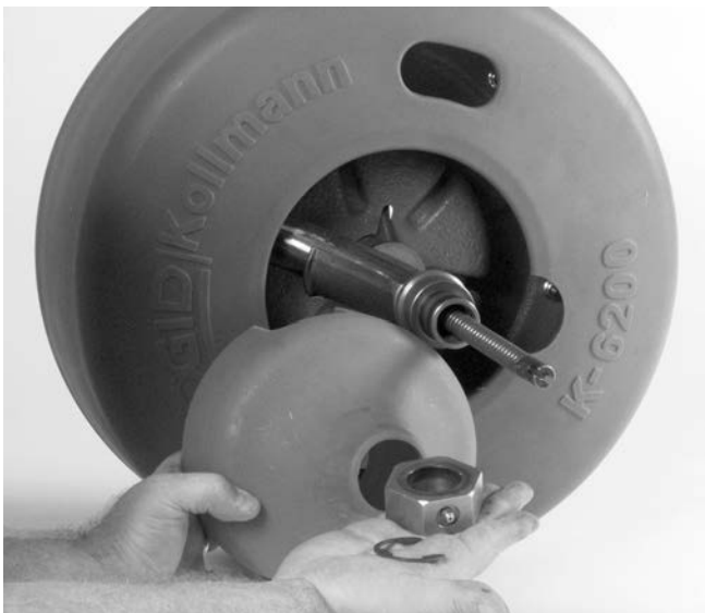
Figure 13 – Remove Retaining Ring and Inner Drum
