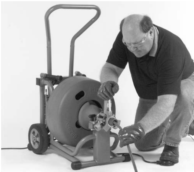
Figure 8 – Proper Operating Position
