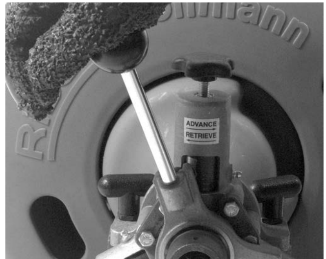
Figure 9 – Feed Lever Operation
