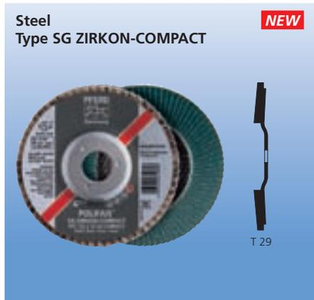
COMPACT flap discs are produced with more material in the same amount of space as typical flap discs. This results in faster grinding performance and increased service life without sacrificing flap grinding performance on edges.
