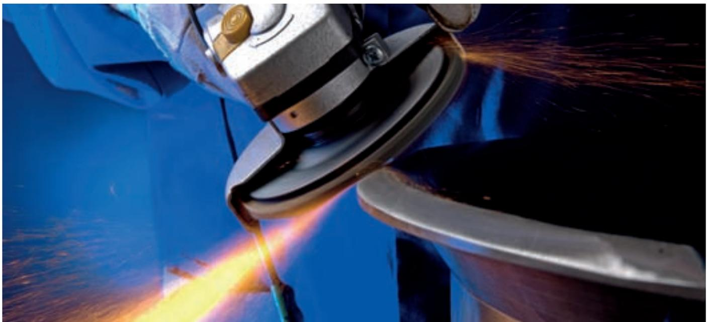
Performance Ceramic POLIFAN® SG-CO is designed for demanding grinding applications on materials which are hard to work. These discs offer highly-aggressive stock removal and high productivity.
