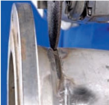
Performance notching pipeline wheel features long service life for reduced wheel changes, fast grinding and cutting of root pass, and excellent edge-holding characteristics.
