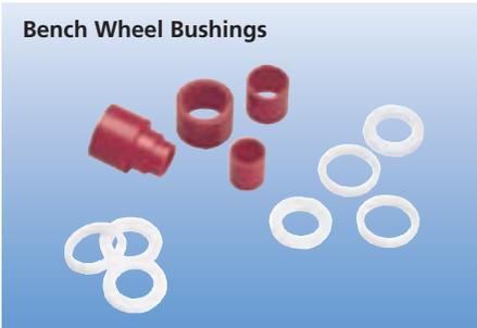
PFERD bench grinder bushings provide a safe method of reducing the wheel arbor to accommodate various spindle sizes. The bushing should be flush on both sides of the wheel, and should not interfere with the flanges.
