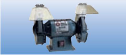
Vitrified bench grinding wheels are offered in aluminum oxide and in green silicon carbide in a wide selection of sizes and grits.
