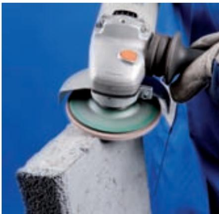
This uncommon flap disc offers a unique solution for applications where surface finish demands are higher than can be achieved by conventional silicon carbide grinding and cup wheels. Designed for grinding on hard to machine metals, plastics and masonry products.
