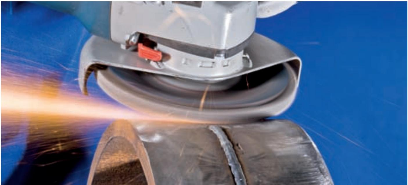
POLIFAN®-CURVE is a PFERD innovation designed to quickly achieve a smooth, consistent surface finish on fillet welds.
