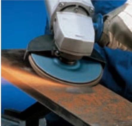
Versatile flap disc for multi-purpose grinding tasks. Suitable for angle grinders of all power outputs. Offers aggressive grinding performance and a good service life. Optimizes inventory management due to its suitability for many materials.
