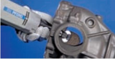
PFERD cones and plugs for horizontal and straight grinders are ideal for cleaning welds and castings. They can be used for internal grinding, blending contours, working in confined areas, and grinding and smoothing weld fillets and corners. High performance for grinding and snagging welds and castings on ferrous materials.
