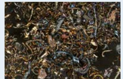
Chips produced with conventional grinding wheels or flap discs. Blue colouration due to overheating.
