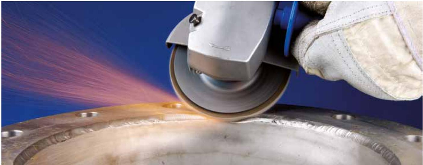
Highly durable flap disc for demanding applications. Premium zirconia coated abrasive material provides sustained high stock removal rates throughout the long disc service life.
