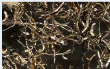
Long chips generated with the POLIFAN®-STRONG-FREEZE. No blue colouration due to low thermal loads.
