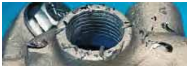
Damaged Threads / Filets endommagés
