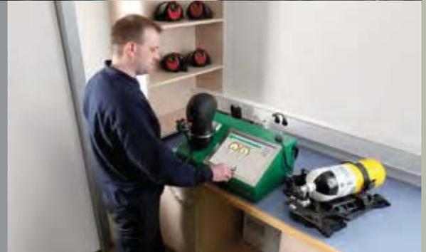
MSA offers a variety of test benches for your workshop with manual or automatically recorded test results. From the mobile test case Multitest to the stationary computer supported test bench smartCHECK, your equipment will be tested to the highest professional standards.
