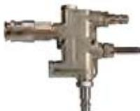
The ASV connects a compressed airline to an SCBA cylinder. This ensures a continuous supply of air in case the external air source (e.g. factory airline) fails.
