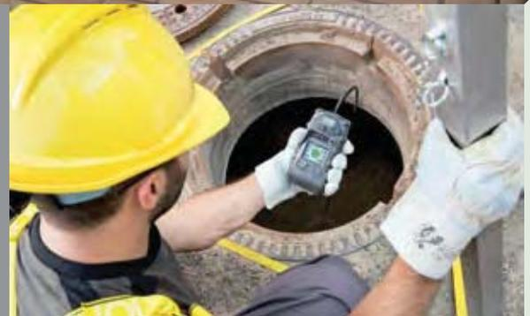
Battery-powered, direct-reading portable instruments are classified into two groups - single-gas instruments or multiple-gas instruments. Depending on the capabilities of the instrument, monitoring can be conducted simultaneously for oxygen and combustible gas, or for oxygen, combustible gas and toxic gases. These devices are commonly referred to as 2-in-1, 3-in-1, 4-in-1 or 5-in-1 alarms.
