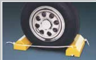
**ROPE LOCK SYSTEM** The original military style chock-to-chock rope lock system allows a wheel chock to be temporarily and securely attached to the opposing wheel chock on the opposite side of the aircraft tire. This chock-locking system ensures that wheel chocks remain firmly positioned against each side of the aircraft tire during engine test procedures.
