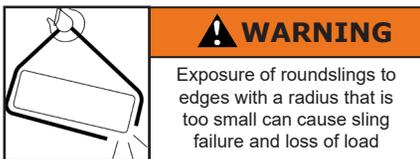
Edges do not need to be "sharp" to cause failure of the sling. Table 3-1 shows the minimum allowable edge radii suitable for contact with unprotected roundslings. Chamfering or cutting off edges is not an acceptable substitute for fully rounding the edges to the minimum radius. Slings can also be damaged from contact with edges or burrs at the sling connection.
