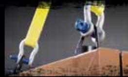
**Four-point crane lift system** facilitates center-point rigging to hoist more safely than with two-point/bar lift systems providing 2500 lbs. gross weight load capacity.
