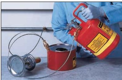
Grounding with antistatic wires
