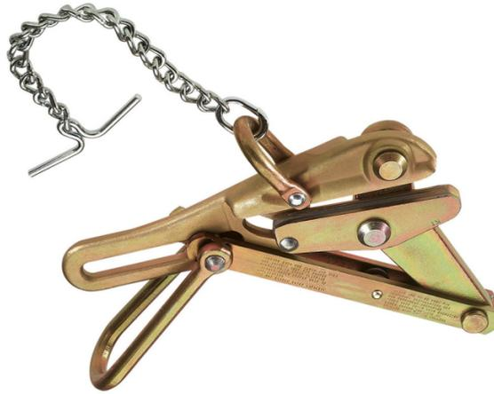
The Klein Tools 1628-16AT Chicago Grip is identical to a Bell-System type -InchH-Inch Strand Puller. It is equipped with a chain, toggle and shackle to keep the grip from falling off the cable. All Klein grips are manufactured from custom drop-forged steel that is machined and heat treated for excellent durability. Each grip is individually hand inspected and actuated for proper function. Grips are also rigorously tested and pulled to rated load to ensure the highest quality and reliability.
