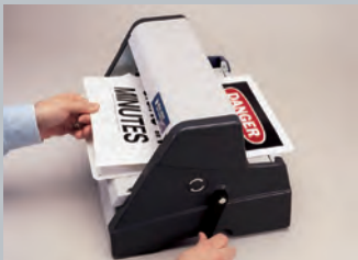
Step 2: Insert sign into laminator and rotate handle until first 1" of sign is "pinched".
