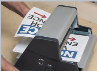
Step 1: Peel away the first 1-1/2" of liner from the back of PowerMark™ printer output. Apply to blank panel, aligning edge of label with edge of panel.
