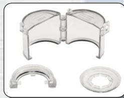
**S2151** - Removable Button & Switch Cover, clear base & cover allow visibility of nameplates & labels. Horseshoe-shaped retrofit base allows use with raised nameplates & off-center installation to accommodate rotary switch knobs. Accommodates button up to 2" (50mm) dia. & 1-3/4" (45mm) tall, Patent pending
