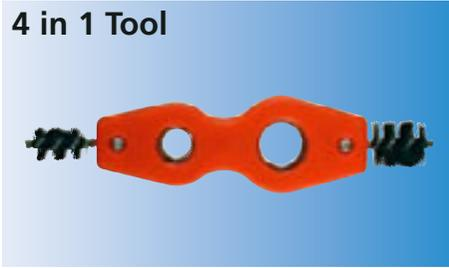
Cleans tubes and fittings inside and outside. Apply to soldering prep, deburring, drill hole cleaning and cleaning battery terminals. Inside diameter 3/4" and 1/2", tube outside diameter 7/8" and 5/8".
