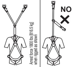
Arrest force: 1800 lbs (816.5 kg) when rigged as shown
