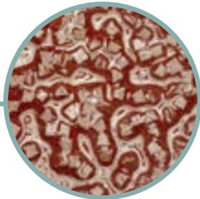
Newly designed 3M precision shaped agglomerate belt for deburring, centerless grinding, cylindrical grinding and flat finishing offers you unprecedented performance on a wide range of metals including carbon steel, stainless steel and other alloys – for outstanding quality, throughput and cost savings. Long lasting abrasive technology helps you achieve desired dimensions and finishes – right from the start!
